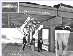
Fig. 1. Passive RFCs are mounted on or embedded within structures. A sensor with antenna is pictured in the upper left-hand corner. The sensor is approximately 90 mm in length. The sensor is interrogated using a pulse/echo technique. The sensor is passive and does not require any local power, such as a battery.
