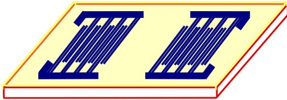
Figure1. Scheme of the Love-wave based delay line
