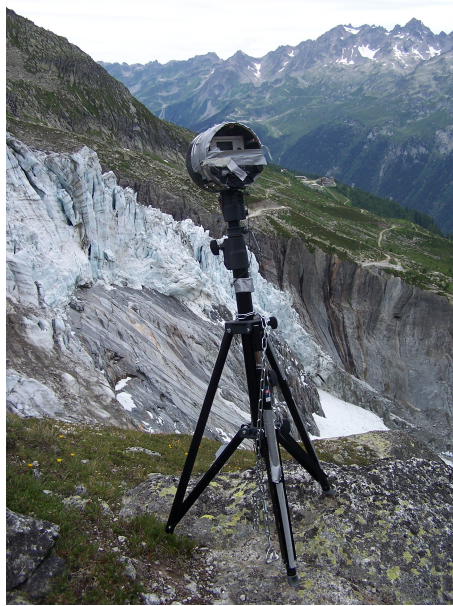
Figure 2: Automated digital camera installed near the Argentière glacier in the summer of 2008.
