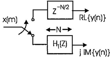
Figure 8.14 Two-path Commutator -driven Hilbert Transform Filter
