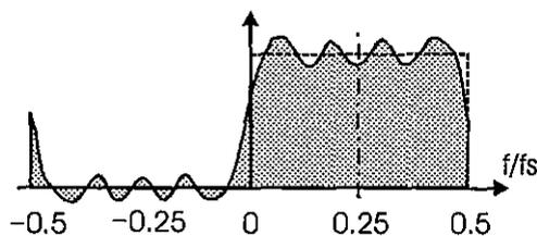
**Figure 8.9** Spectral Characteristics of Hilbert Transform Half-band Filter
