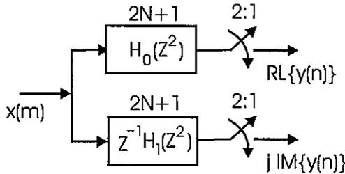
**Figure 8.12** Two-path Model of Hilbert Transform Filter with Complex Impulse Response
