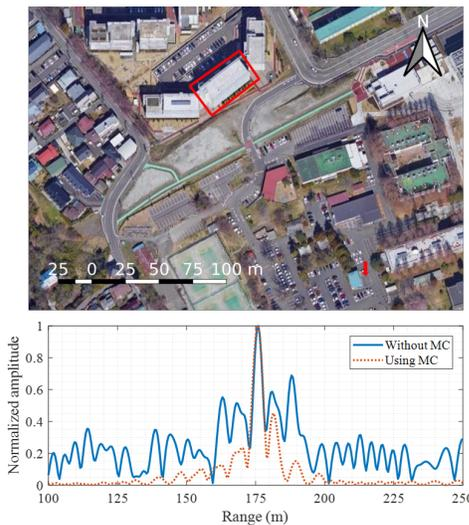
Fig. 19. Building detection results with and without MC based gap filling.
