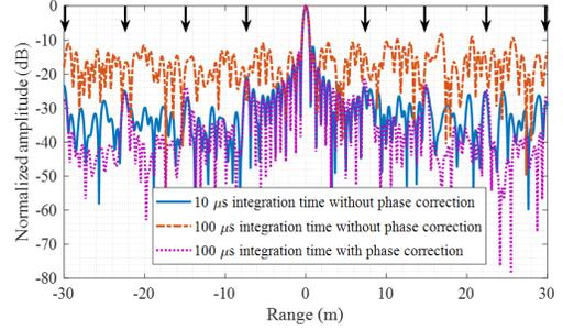
Fig. 13. Estimated time delay between two co-located antennas using ISDB-S signal with different integration time in dB scale.
