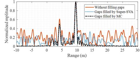
Fig. 20. Detection of two metallic plates with ISDB-S signal by different gap filling methods with an integration time of  $10 \mu s$ .
