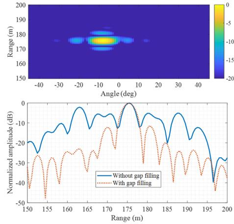
Fig. 23. Top: 2D focused image of the high building obtained by the proposed spectral gap filling method. Bottom: Comparison between Fig. 23 and Fig. 22 in the range direction at  $-9^\circ$ .
