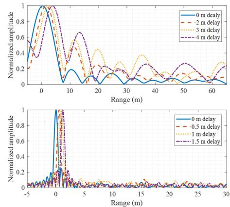
Fig. 10. Estimated time delays between two antennas using an inverse filter. Top: ISDB-T signal. Bottom: ISDB-S signal. Integration time is 10  $\mu$ s.
