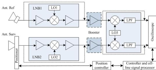
Fig. 7. Block diagram of the designed PBR system.
