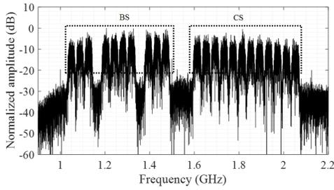
Fig. 5. Spectrum of ISDB-S signal in Japan. BS and CS are broadcast by different satellites. The local oscillation frequency of LNB is 10.678 GHz.
