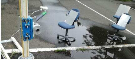
Fig. 16. Detection of three metallic plates with the surveillance antenna sledded on the positioner with a 5 mm step.
