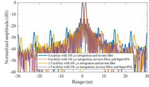
Fig. 14. Estimated time delays with and without using Super-SVA.
