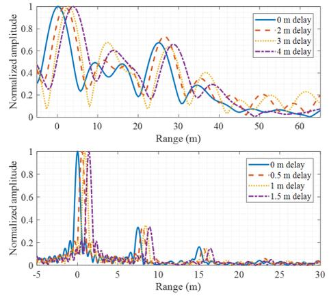
Fig. 9. Estimated time delays between two antennas. Top: ISDB-T with four different distances (0m, 2m, 3m, and 4m). Bottom: ISDB-S with four different distances (0m, 0.5m, 1m, and 1.5m). Integration time is 10  $\mu$ s.
