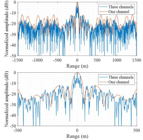
Fig. 3. Ambiguity function of three ISDB-T TV channels with an integration time of 10  $\mu s$ . The bottom sub-figure is the zoomed version of top sub-figure.
