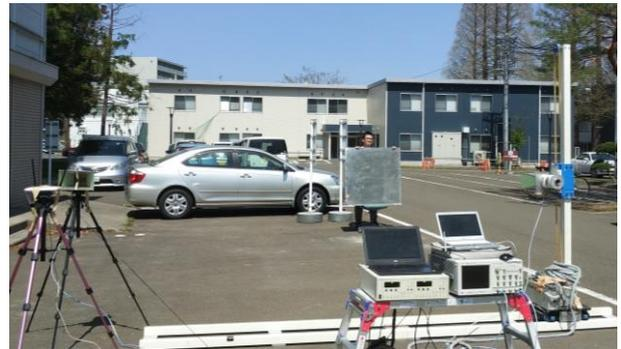
Fig. 6 Experiment setup for passive bistatic SAR imaging.
