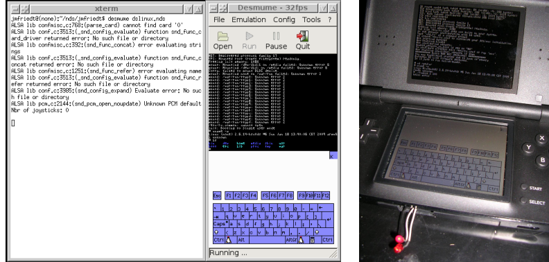
Figure 1: Left : DSLinux running on the desmume NDS emulator. Right: the same result is obtained on the console, here shown with the modified rumble pack cartridge for controlling LEDs (section 1.2).
