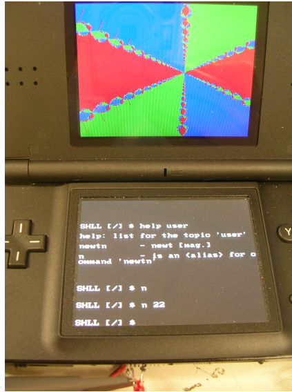
Figure 9: A new RTEMS command ( newtn ): calculation and drawing of Newton's fractal, used as an opportunity to illustrate the software emulation of floating point calculation and accessing the framebuffer display.
