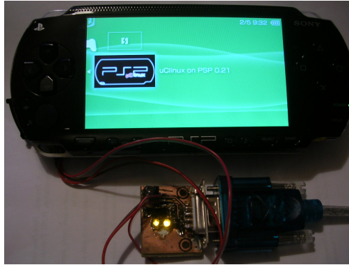
Figure 12: The most convenient communication interface with the PSP: the asynchronous serial port next to the audio connector is compatible with RS232. uClinux will be loaded as a game over Sony's operating system, so the native functions for accessing hardware peripherals are only available to the bootloader but no longer once uClinux is loaded.
