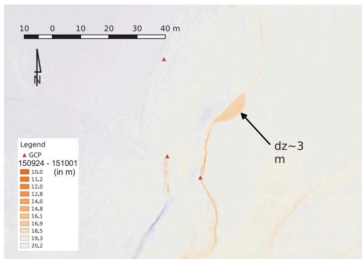
**Figure 10.** Difference of DEM (DoD) for assessing moraine movements due to a significant flood event, with one wall of the canyon collapsing between the two dates. The images for generating the DEMs were acquired on 24 September 2015 and 1 October 2015. The landslide generated canyon collapse depth is about 3 m.
