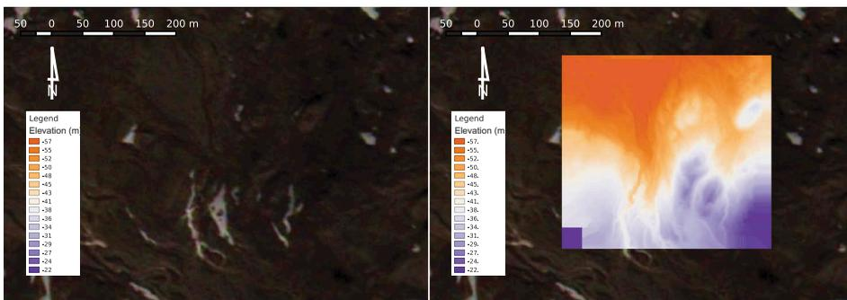
**Figure 9.** (Left) Formosat image acquired on 22 July 2009 of the area of interest. (Right) Overlap of a DEM acquired on 24 September 2015 of the same region, illustrating the consistency and fine hydrological network visible on the topography. The average tilt on the DEM has not been compensated for: water flows from bottom to top.
