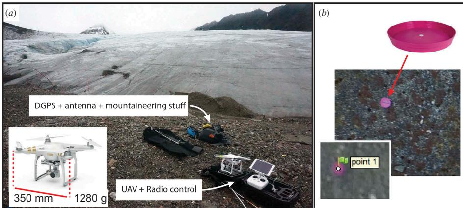
**Figure 5.** A well-suited package for SfM survey in Arctic/mountain terrain and cold regions. All equipments are easily packable in a backpack and makes travel into the moraine and work easier (a). Pink gardening saucers are perfect GCPs since the environment is monotonous (b).
