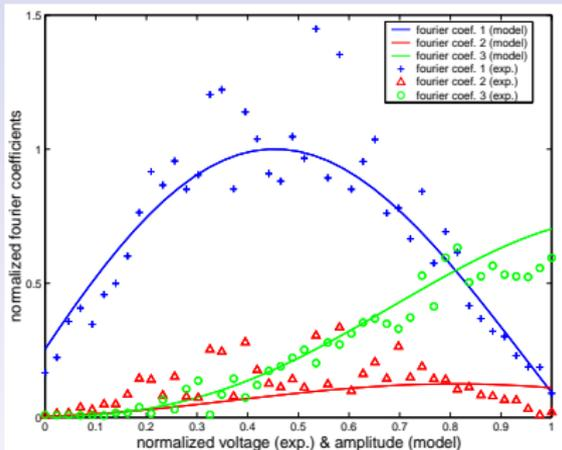
abscissa is graduated in voltage from 400 to 9000 mV (experimental data), which is also equal to (simulated data) a vibration amplitude of  $\lambda/21 = 23$  nm to  $\lambda/1.7 = 290$  nm ( $\lambda = 488$  nm in this experiment).
