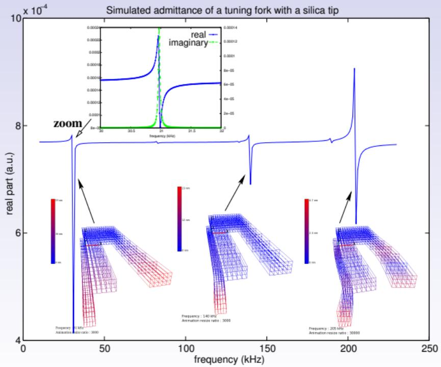
Quartz tuning fork vibration amplitude as a limitation of spatial resolution of shear force microscopes
