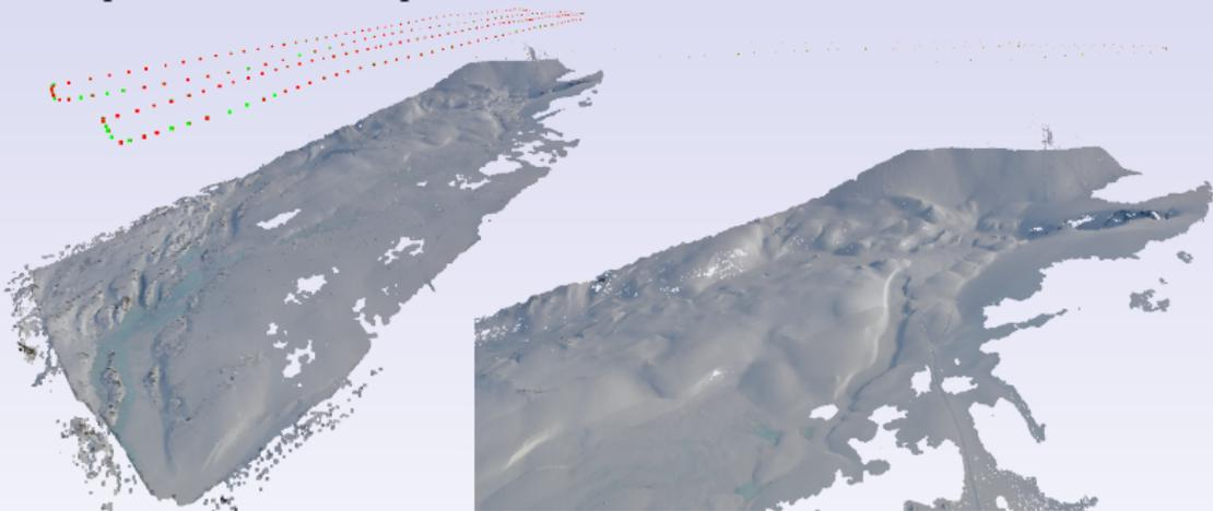
Camera position consistent <sup>3</sup> with flight path: we can continue processing.
