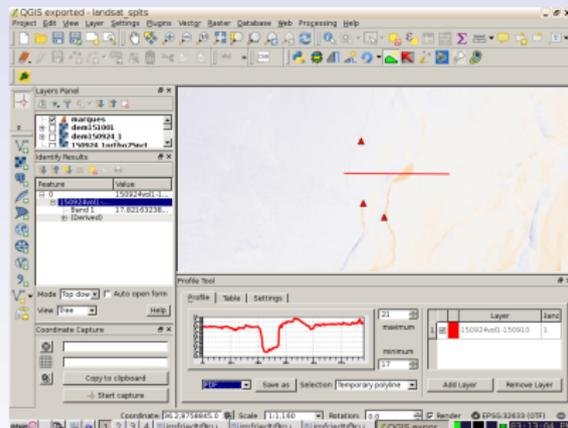
⇒ collapse of 3-m deep canyon wall within 1-week of repeated DEM measurement, consistent with observations on the field
