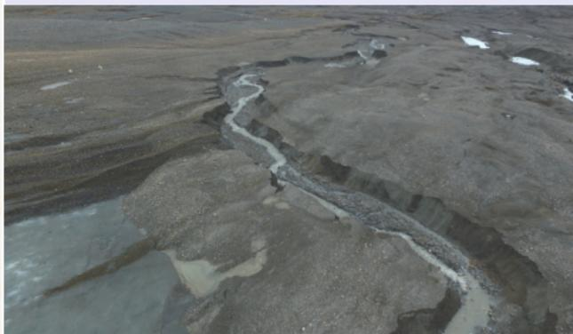
⇒ collapse of 3-m deep canyon wall within 1-week of repeated DEM measurement, consistent with observations on the field
