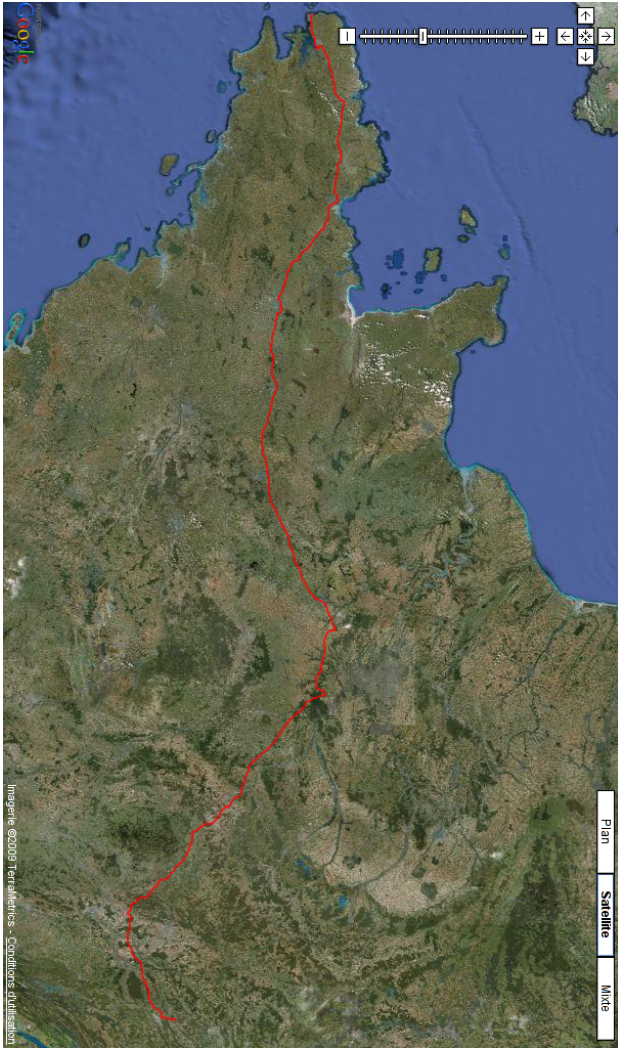
Figure 9. Example of storing a GPS track onboard a moving vehicle – incompatible with low-power radiofrequency data transmission – driving from the west to east of France – a total of 9.2 MB stored during the 11 hour trip. The red track is an overlay over the satellite view of the path followed during the trip.
