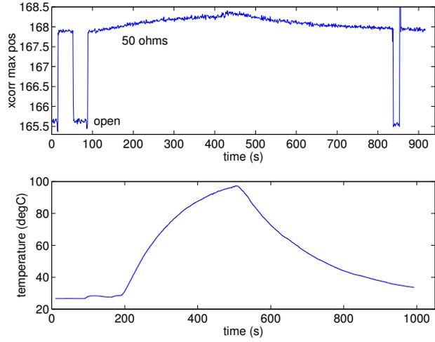
FIG. 8. The device used earlier (Fig. 6) as a dipole was used as a 4-pole coupled oscillator. The second port was either loaded by a  $50 \Omega$  load, or opened. The switch behavior probed through a wireless link is dominant over the temperature variation in the 20-80  $^{\circ}\text{C}$  range.
