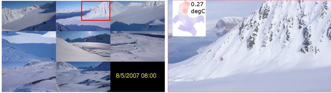
Figure 4.2: Top left: mosaic of pictures taken at the same time by 8 automated digital camera located around the glacier basin under investigation. Top right: the use of high resolution digital camera allows for zooming on regions of interest, here a slope for analyzing the snow cover and dynamics of snow accumulation from the slopes to the glacier.
