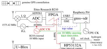
40 MHz is 4-times multiplication of reference 10 MHz input of B210 HM always clocks the HP53132A counter and might clock the B210  $\,$
