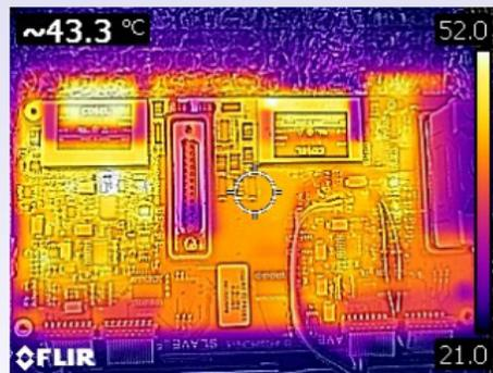
Operational amplifier rises to > 50°C, inducing offset and drift in surrounding passive components
