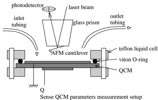
Fig. 4. Experimental setup of the combined QCM and AFM instrument, based on a commercial AFM designed by molecular imaging and a QCM parameter analysis instrument built by Q-Sense AB (Göteborg, Sweden).
