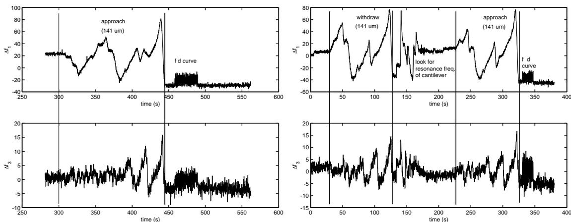
Fig. 5. Graphs displaying the effect of longitudinal waves on the frequency stability of the resonator (top graphs show the evolution of frequency of the first mode, bottom graphs show the evolution of frequency of the third mode). Total displacement during cantilever approach is 141  $\mu\text{m}$ , which is quite close to the theoretical half-wavelength of an acoustic wave propagating in water at 5 MHz (152  $\mu\text{m}$ ).<sup>4)</sup>
