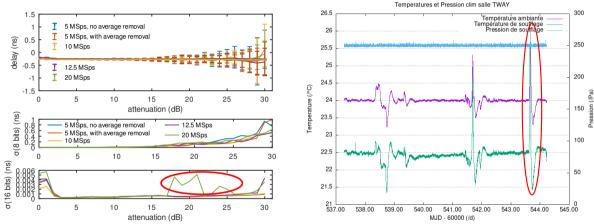
Huge impact of temperature (red ellipses) Need to keep **all 14 bits** for best PRN timing capability (time resolution improvement = synchronization signal SNR)
