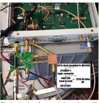
Clock shaping from unbalanced to differential using a zero-crossing detector (LTC6957-1)
