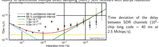
1. Ability to synchronize multiple direct sampling (ADC) SDR receivers with sub-ps resolution <sup>4</sup>
