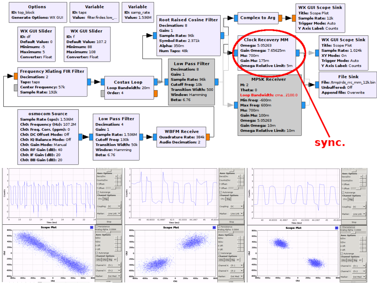
Figure 14: Top: signal processing chain, with the addition of the bitrate synchronization blocks following the carrier synchronization (Costas). Bottom: constellation diagrams (XY mode oscilloscope fed with complex data) for various processing conditions – from left to right, output of the Costas loop (no bitrate synchronization), bitrate synchronization following a low-pass filter, and finally following and RRC. Two distinct point clouds ensure proper symbol separation.
