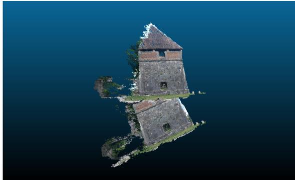
FIGURE 23 – Effect of the camera position altitude uncertainty on the point cloud orientation. The tilted tower results from using raw GPS measurements exhibiting  $\pm 5$  m altitude variations. The “vertical” tower is the result of the same computation, but this time with all altitudes set to the same value for all shots.
