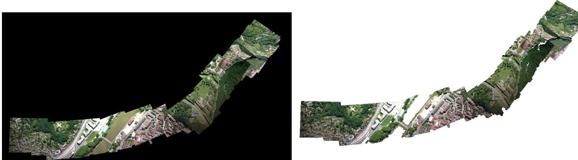
FIGURE 9 – Left : mosaïque of the orthorectified images generated by **Tawny** for defining the color of the pixels in the point cloud (**Ortho-Eg-Test-Redr.tif** file in the **Ortho-** directory provided as argument to **Tawny**). Right : the colored point cloud, azimuthal view. Notice the lack of samples over the river which is associated with a lack of correlation between images.
