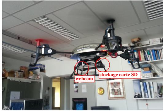
FIGURE 16 – Indoor flight of the drone fitted with its camera
