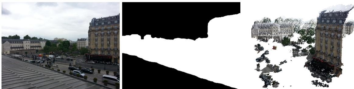
FIGURE 4 – Left : one of the original image used for generating a model of the area surrounding the East train station in Paris. Notice on the foreground the balcony and clouds in the sky which yield a hardly usable point cloud result. Middle : mask removing (black regions) these useless areas. Right : the resulting point cloud when the mask information is used, reducing the point cloud to the region of interest.
