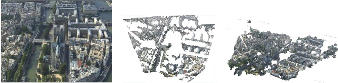
FIGURE 12 – Model of the Paris church Notre Dame and Île de la Cité obtained by processing images extracted from the Paris Vu du Ciel documentary. Left : one of the pictures extracted from the DVD for processing. Middle : azimuthal view of the point cloud, on which Île de la Cité and the largest buildings are clearly visible. Right : oblique view of the same point cloud, allowing the visualization of the two protruding towers of the church.
