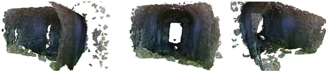
FIGURE 7 – Point clouds of the entrance of Fort des Trois Chalets near Besançon : tunnels provide a favorable geometry for generating point clouds.
