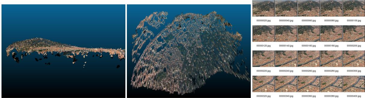
FIGURE 15 – Sète, oblique view demonstrating the topography generated from the pictures extracted from the movie, and azimuthal view. Right : some of the images taken from the movie used to generate the point cloud.
