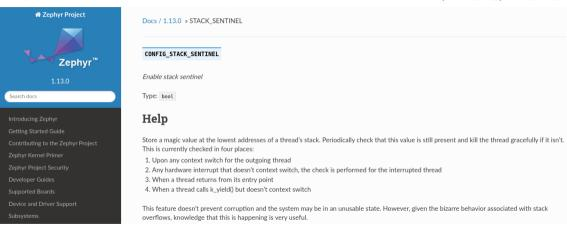
↑ Example of stack debugging functionality provided by Zephyr Project.
