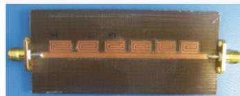
Fig. 3.27 Photograph of 6-bit multiresonator on Taocnic TLX-0
