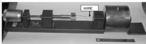
Fig. 14. Displacement sensor was mounted on a displacement test fixture, and a wire rod was attached to the front of the displacement sensor. Using the micrometer, the diaphragm of the displacement sensor was translated in 0.1 mm increments. At each increment the resonant frequency of the cavity was determined using the servo method described.
