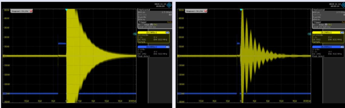
Time-domain characterization of a dual-resonator SAW sensor: left narrowband excitation, right broadband excitation ( $\Rightarrow$  beatnote)
