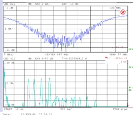
Inverse Fourier transform of frequency sweep: narrow frequency sweep (2 MHz, top left) does not provide enough time resolution. This delay line requires at least 20 MHz bandwidth.
