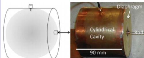
Fig. 13. Displacement sensor employing a corrugated diaphragm on one end with a rod attached. As the rod is displaced, the diaphragm is displaced causing the cavity to change dimension and hence shift the resonant frequency. The cavity is 100 mm in diameter. An SMA connector-wire probe is used to couple signals in and out of the cavity.
