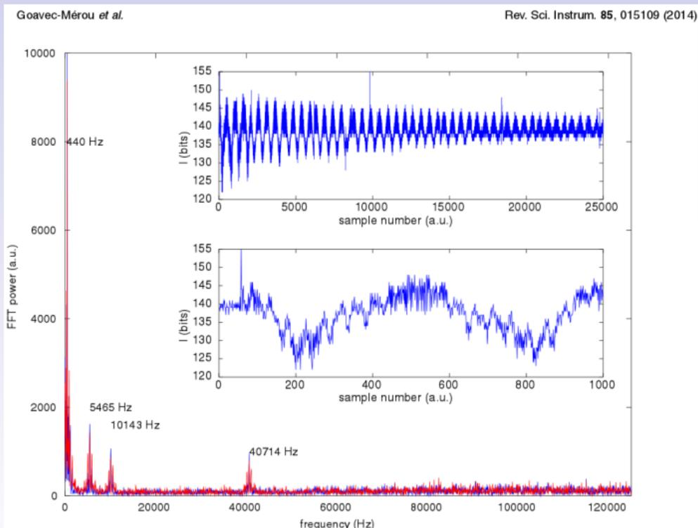
Impulse response: mode distribution **consistent** with acoustic (audio card) and optical measurements
