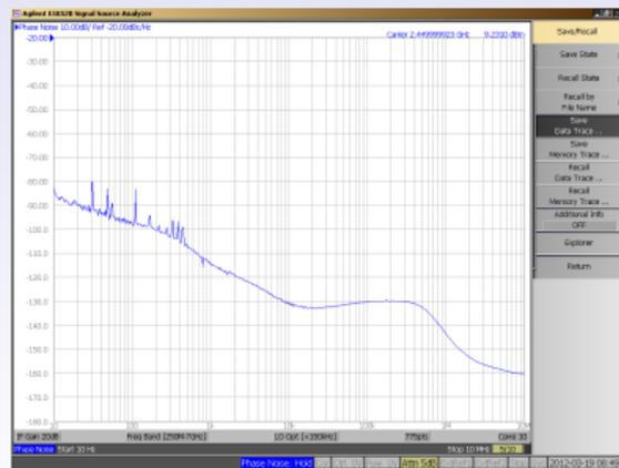
2.45 GHz source generated by an Analog Devices ADF4360-0 Phase Locked Loop (poorly controlled), & Rohde & Schwartz SMA 100 A tabletop frequency synthesizer.
