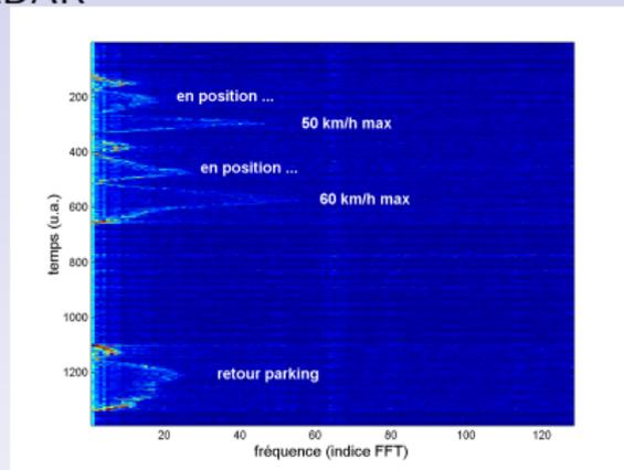
Target velocity induces frequency shift  $f_D = 2 \times \frac{f_0 v}{c}$  when  $v \ll c$
