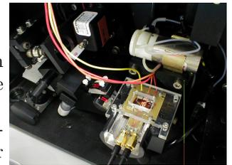
Experimental setup applied to electrodeposition of copper
