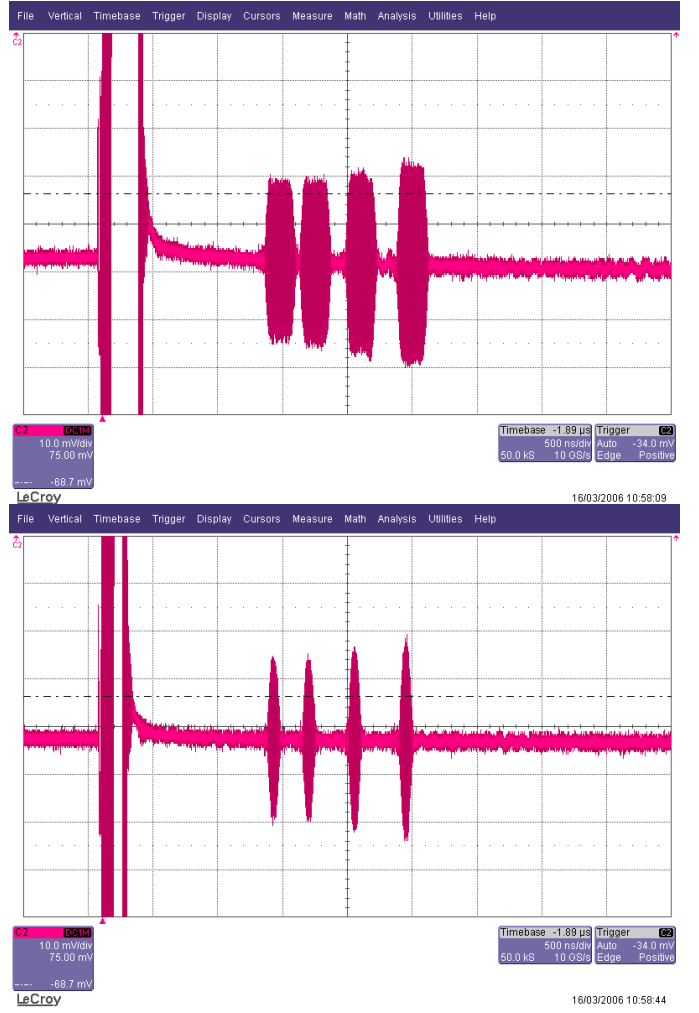
Fig. 4. Two examples of echos observed on the delay line reflection signal, as a function of excitation pulse length. Too long a pulse blurs the echos and makes the identification of the time delay more difficult, without increasing the reflected signal level: this experimental result is consistent with the matched filter theory which states that the optimal number of periods is equal to the number of interdigitated fingers in the transducer. The hardware used in this experiment is unable to generate an excitation pulse with less periods than the number of interdigitated fingers in the transducer of the delay line.
