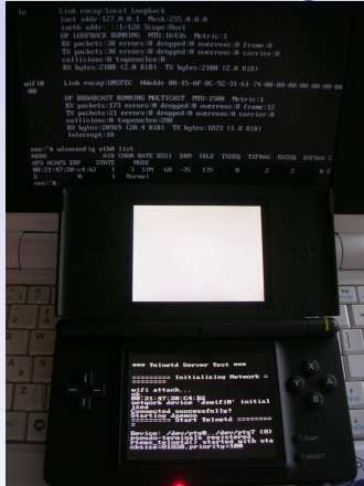
Direct connection from NDS to eeePC configured as AP 3
