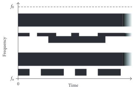
FIGURE 5: FDMA/TDMA signals over the time/frequency plane, spectrum pool.
