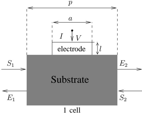
Fig. 5. Definition of the elementary cell of a mixed matrix model
