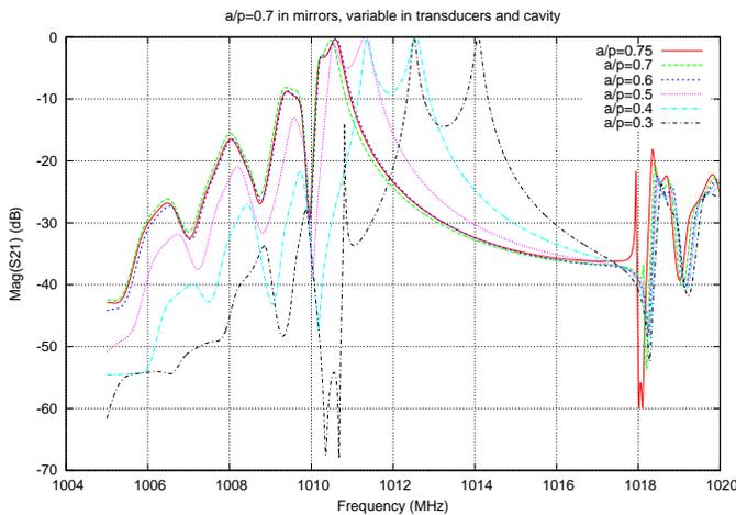
Fig. 7. Simulations of the response of STW quadrupole resonators in which the  $a/p$  ratio is kept equal to 0.7 in the mirrors and varied in the transducer and cavity.
