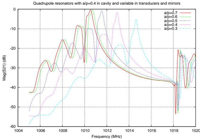
Fig. 6. Simulations of the response of STW quadrupole resonators in which the  $a/p$  ratio is kept constant over the mirror and transducers but varied in the cavity region (5 finger pairs). We notice that the cavity hardly affects the shape of the response which is thus representative of the synchronous device configuration.
