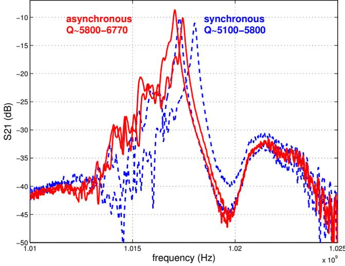
Fig. 4. Experimental measurement of quadrupole synchronous and asynchronous resonators insertion loss (magnitude of  $S_{21}$ ).
