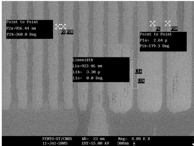
Fig. 2. Scanning electron microscope images of a synchronous device (the mirror is to the left of the image and the interdigitated transducer to the right).
