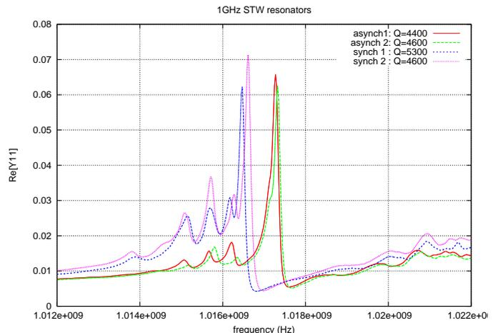
Fig. 3. Comparison of the measured admittance (real part) of synchronous and asynchronous two-port resonators. Although the asynchronous design displays less ripples out of the pass-band frequency range – making them suitable for narrow-band filtering applications – they display a lower quality factor than the synchronous design – making the latter more suitable for oscillator applications.
